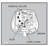
The wire coloured green and yellow must be connected to the terminal marked with the letter «E» or by the earth symbol  $\frac{1}{=}$  or coloured green and yellow.
